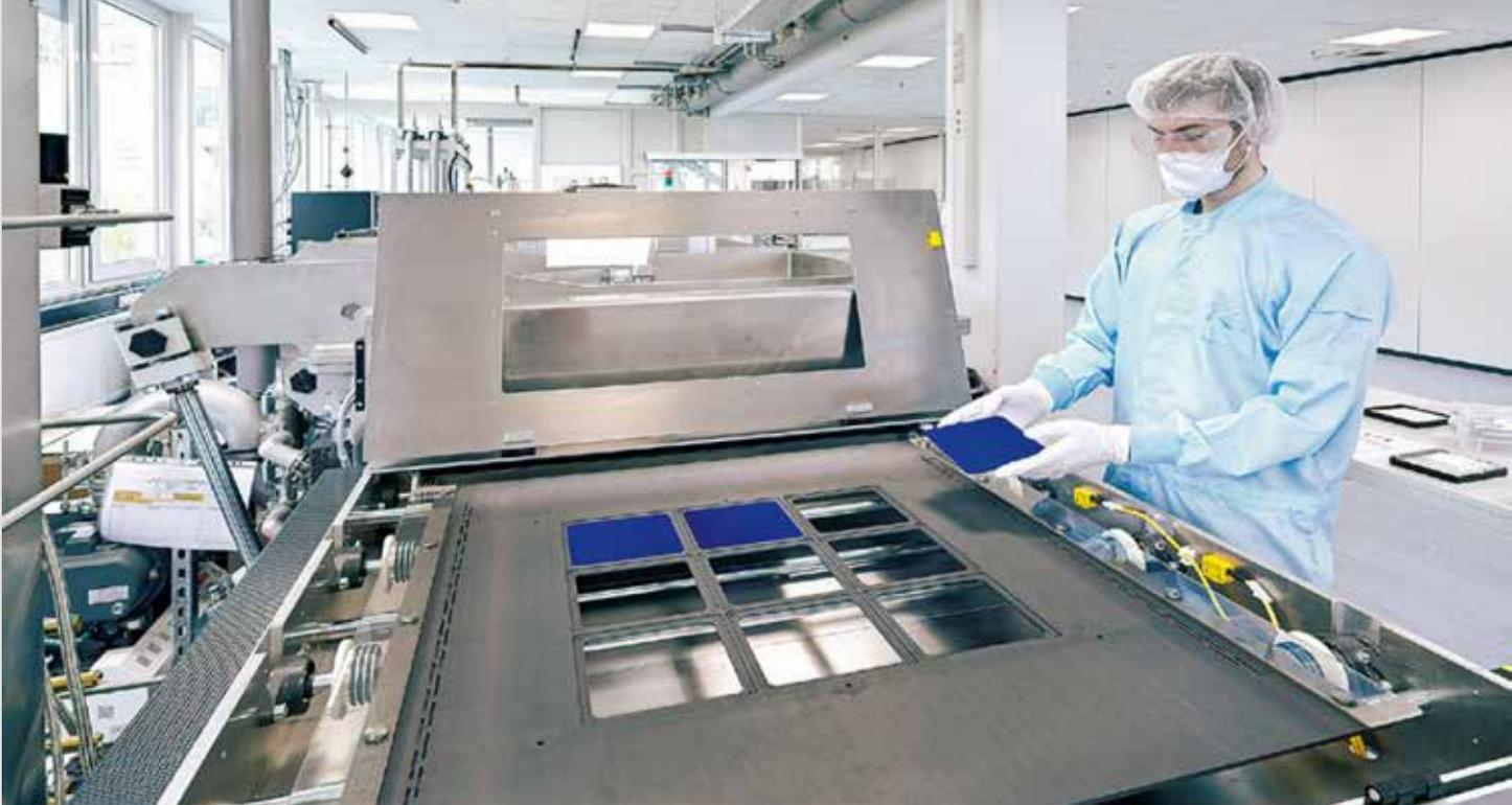
PVD deposition tool with wafers after TCO deposition.
