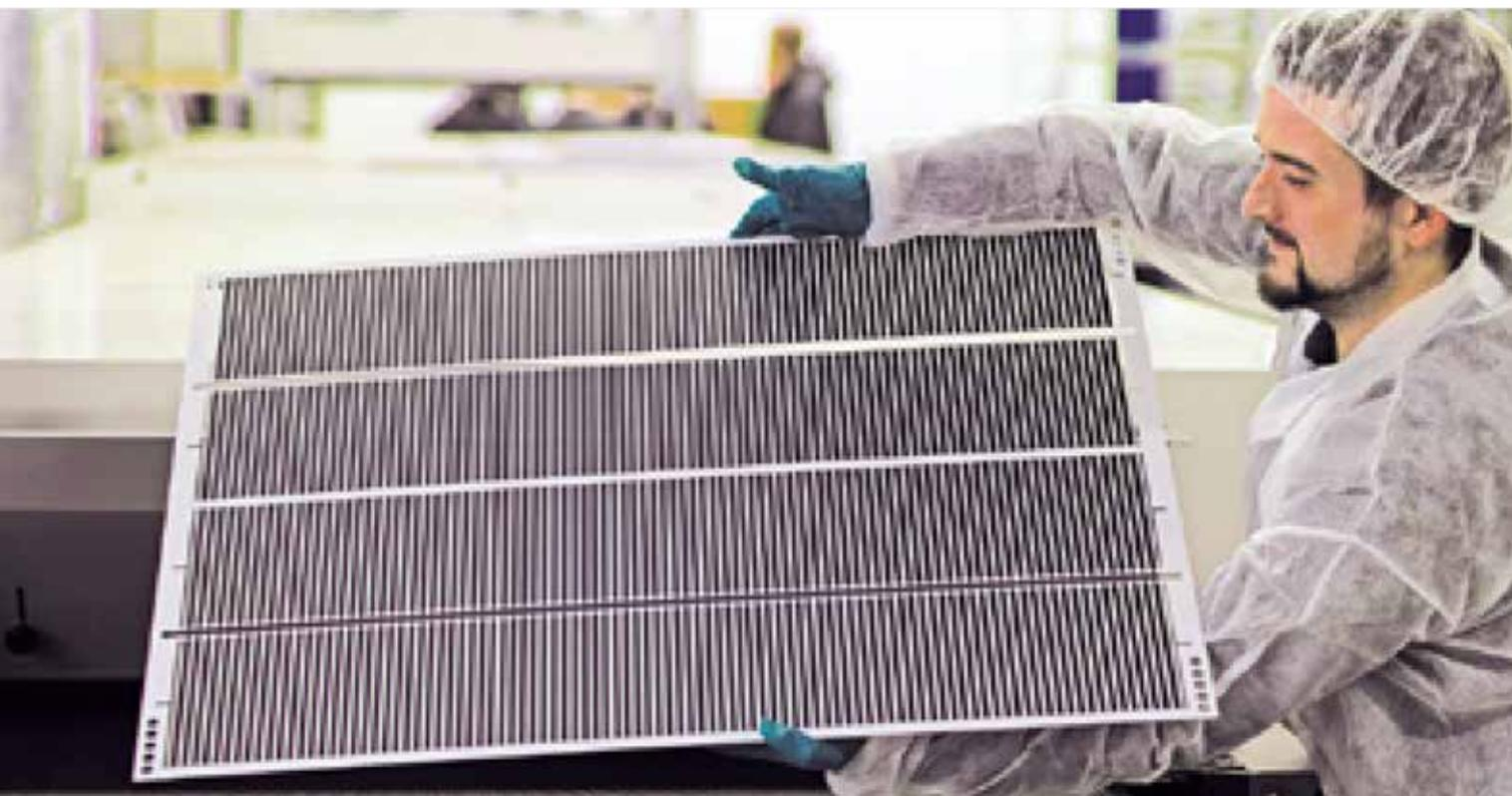
*Screen-printed photoelectrode of a perovskite solar module.*
