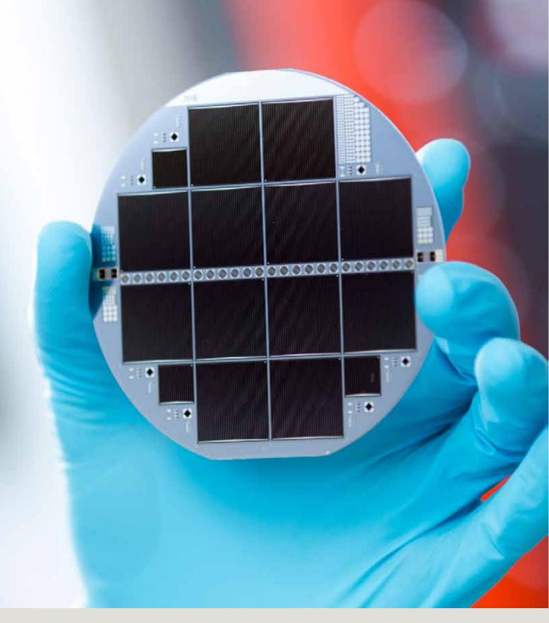
Multi-junction solar cell of III-V semiconductors and silicon, which converts 33.3 % of solar radiation into electricity. By comparison, the best conventional silicon solar cells to date achieve an efficiency value of 26.7 %. The higher power is enabled by fifteen very thin III-V semiconductor layers, which have a total thickness of only 0.002 mm. The entire solar cell is approx. 0.25 mm thin. The III-V layers convert the visible part of the solar spectrum particularly efficiently.
