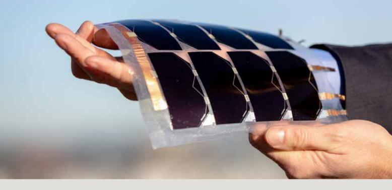
Ultra leight PV module with high efficiency. GalnP/GalnAs/Ge triple-junction solar cells.
