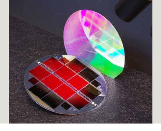
The new III-V // silicon tandem solar cell with 35.9 % efficiency. The top subcells, made of GalnP, glow red under illumination. This is a sign of outstanding material quality. The back side of the cell shimmers in rainbow colors, because a nanostructure was used on this side to increase the efficiency.
