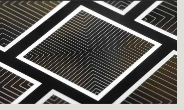
The TOPCoRE solar cell achieved 26 percent efficiency, a new world record for both-sides-contacted solar cells.
