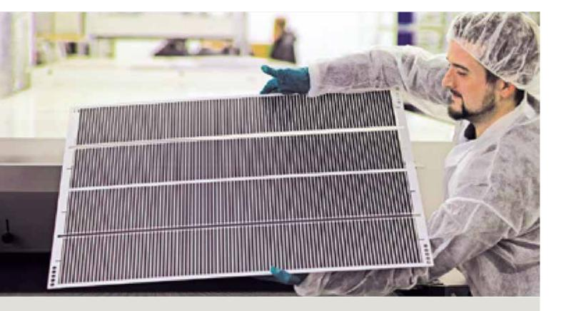
Screen-printed photoelectrode of a perovskite solar module.
