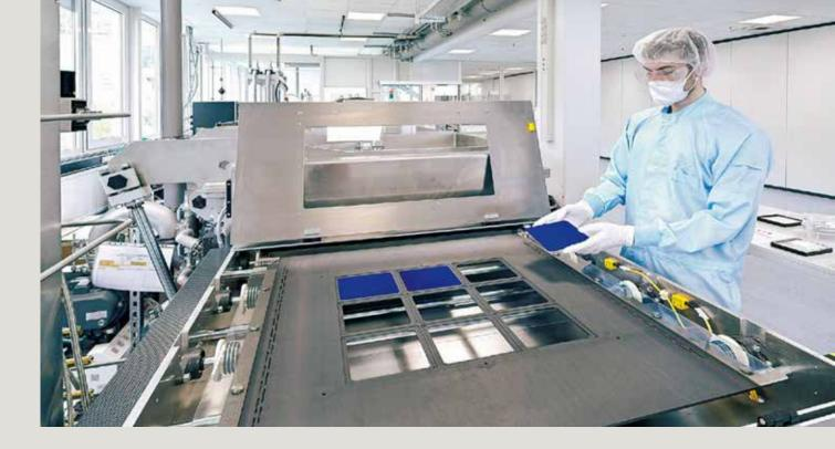
PVD deposition tool with wafers after TCO deposition.
